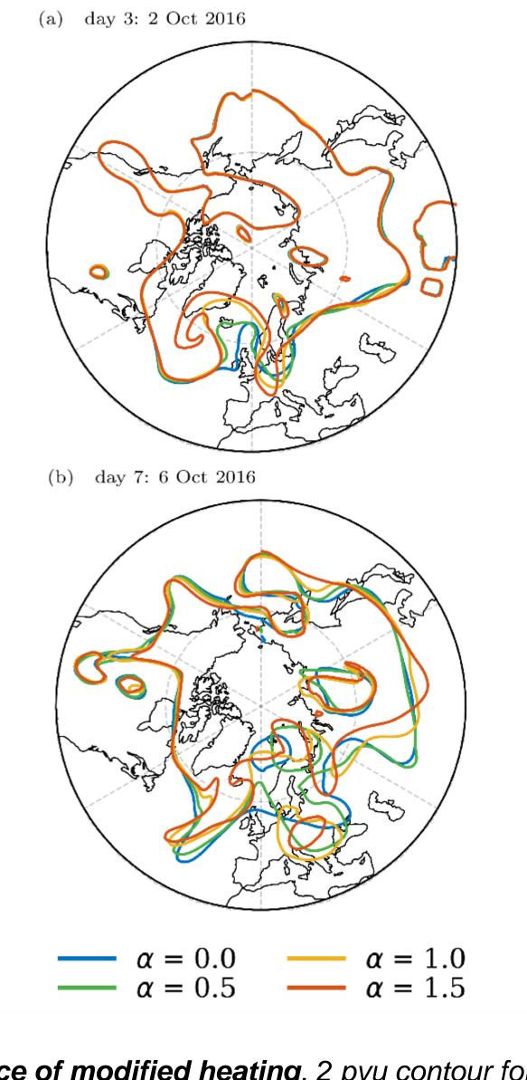
Influence of modified heating. 2 pvu contour for case "Thor" on (a) 2 October 2016 (day 3) and (b) 6 October 2016 (day 7) for different modifications of upstream latent heating (simulated heating is multiplied with a factor α).
